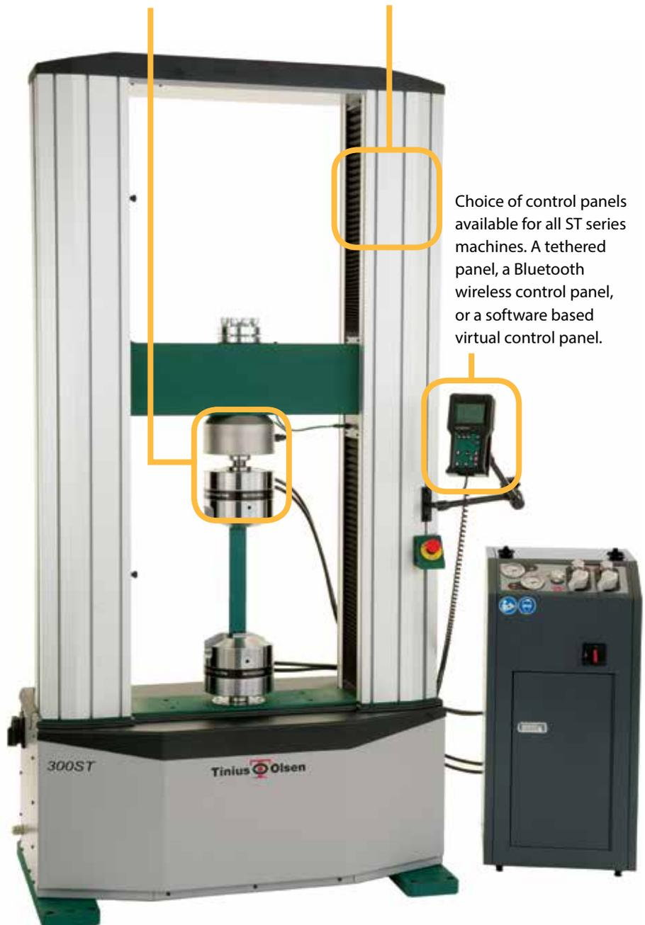
Choice of control panels available for all ST series machines. A tethered panel, a Bluetooth wireless control panel, or a software based virtual control panel.
