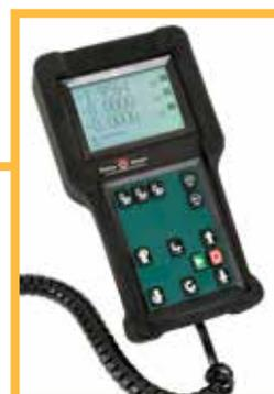
This tethered interface option features larger tactile feedback buttons for the operation of the testing frame; these make it ideal for users who need to wear protective gloves while operating the machine. The display provides simple numerical display of individual channels used on the testing machine.
